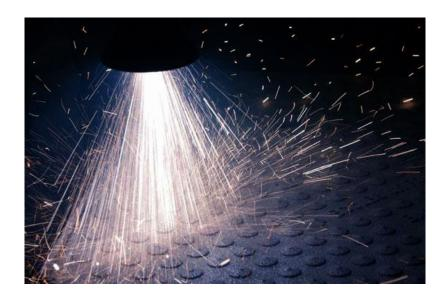
The Metal Spray process can provide engineering coatings including antispark, chrome replacement, non-stick, reclamation, grip, thermal barrier and wear resistance coatings. Each type of coating adds an Engineered Surface which in turn provides Exceptional Performance.
