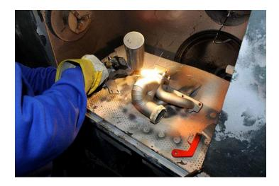
Thermal Barrier Coatings (TBCs) consist of ceramic materials which are widely used on vehicle exhausts, turbocharger casings, heat shields and other vehicle components to reduce heat transfer and improve vehicle performance. TBCs are also used to protect Aerospace metallic components from hydrocarbon combustion. High performance coatings can be used to protect against wear and high temperature corrosion. This is particularly ever present in the Automotive industry; examples are listed below.
